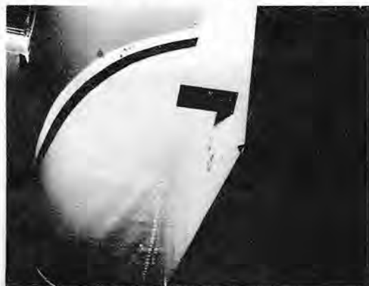
Fig. 4.3 Hole melted in trailing edge corner of ventral fin.
