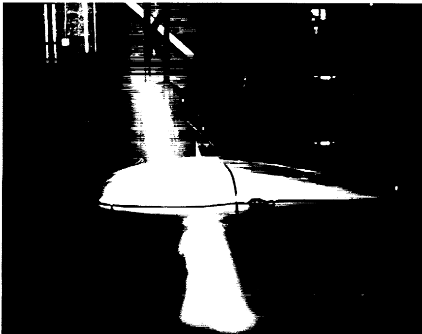
Figure 6.32 Direct strike to unprotected fuel filler cap resulting in internal sparking and ignition of fuel.
